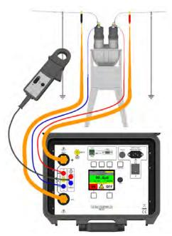
through 20m output leads to reach the contacts of even the largest circuit breakers. Optional lead extensions are available which extend the high current and sense leads by 3, 5 or 10m.
